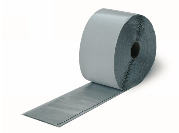
Figure 28. Plasto-elastic butyl rubber adhesive / sealant applied to one side of an aluminised polyester film. Courtesy Tremco illbruck.
